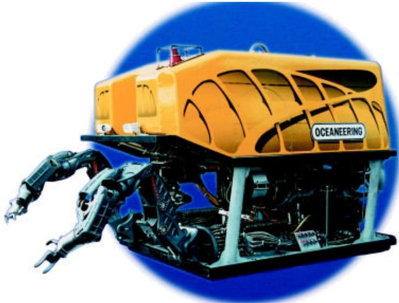
*Left: Oceaneering's deep-sea Remotely Operated Vehicles (ROV's) are used for petroleum exploration and production, communications cable installation and maintenance and recovery operation including the RMS Titanic and TWA Flight 800*
